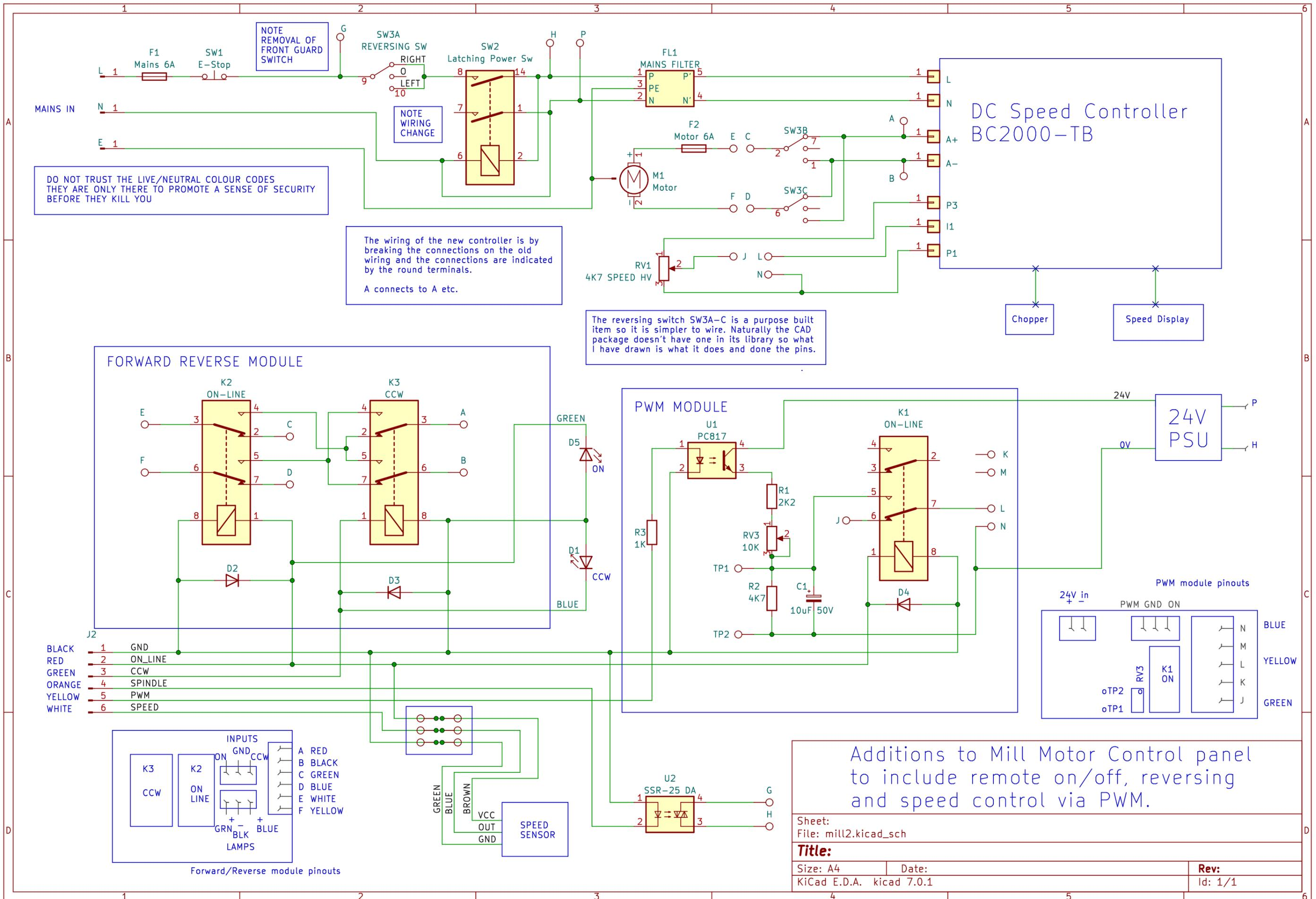
Additions to Mill Motor Control panel to include remote on/off, reversing and speed control via PWM.
