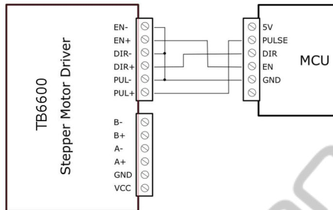
**Note:** When “EN” is in the valid state, the motor is in a free state (Off-line mode). In this mode, you can adjust the motor shaft position manually. When “EN” is in the invalid state, the motor will be in an automatic control mode.
