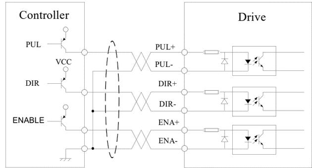
Figure 3: Connections to PNP signal (common-cathode)
