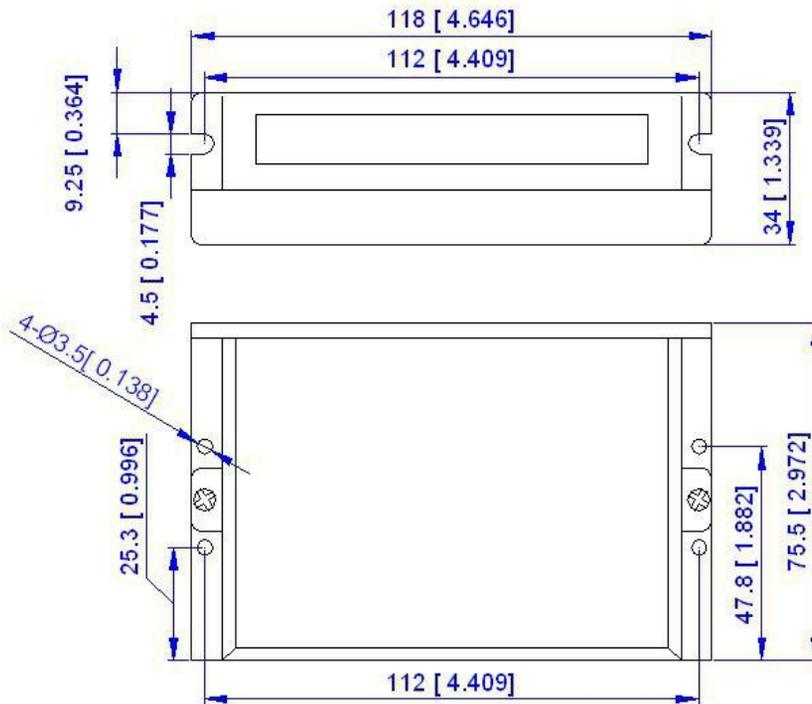
Figure 1: Mechanical specifications
