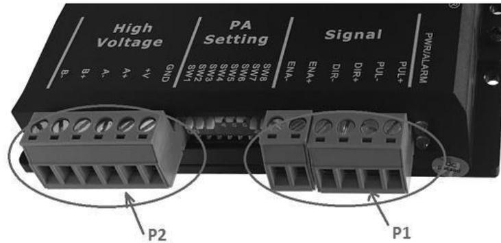
The DM556T has two connector blocks P1&P2 (see above picture). P1 is for control signals connections, and P2 is for power and motor connections. The following tables are brief descriptions of the two connectors. More detailed descriptions of the pins and related issues are presented in section 4, 5, 9.
