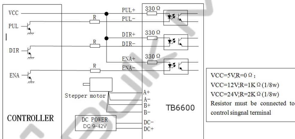
Pulse signal connects to PUL-; direction signal connects to Dir- ; Enable signal connects to EN-. As shown below:
