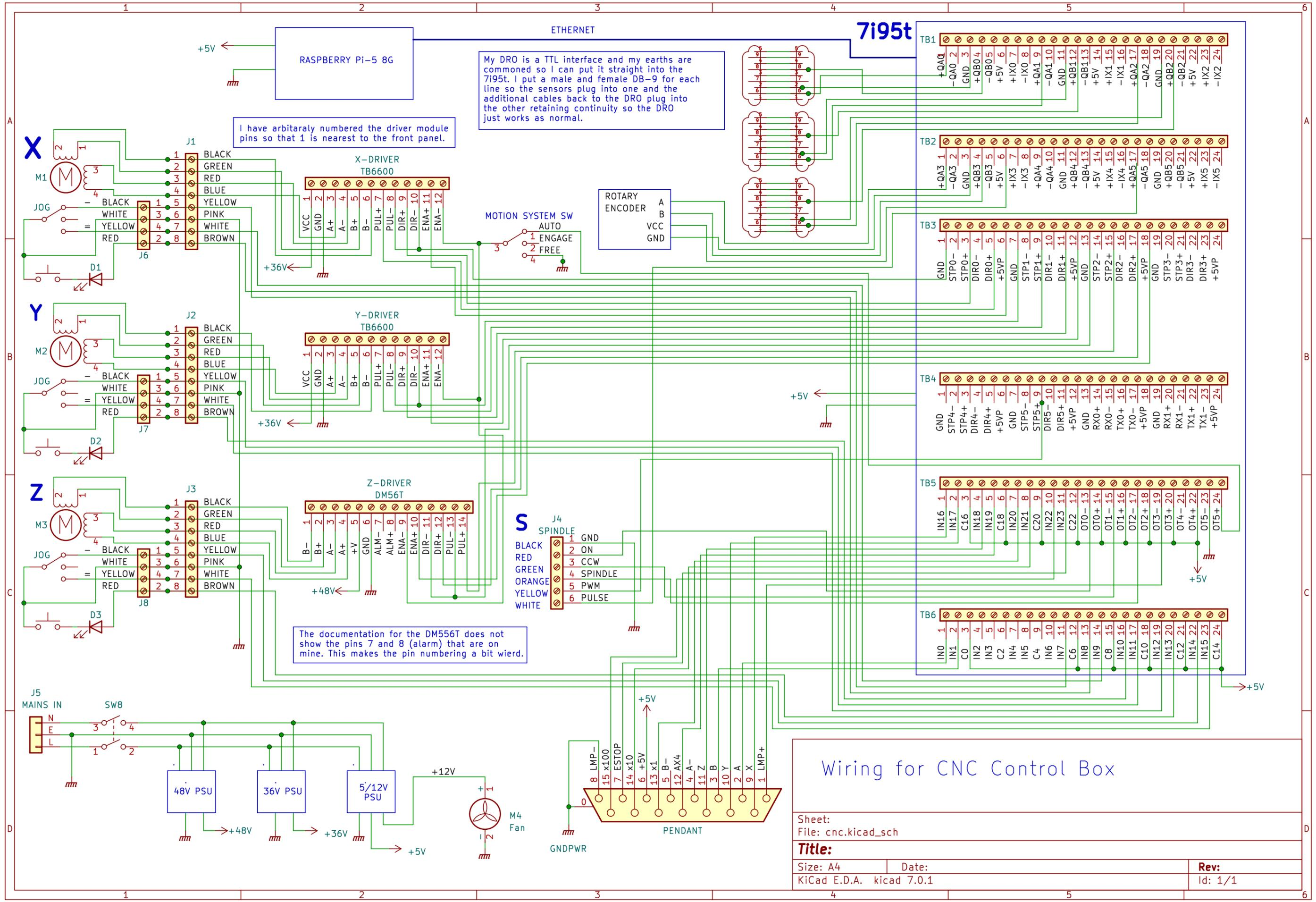
I have arbitrarily numbered the driver module pins so that 1 is nearest to the front panel.
